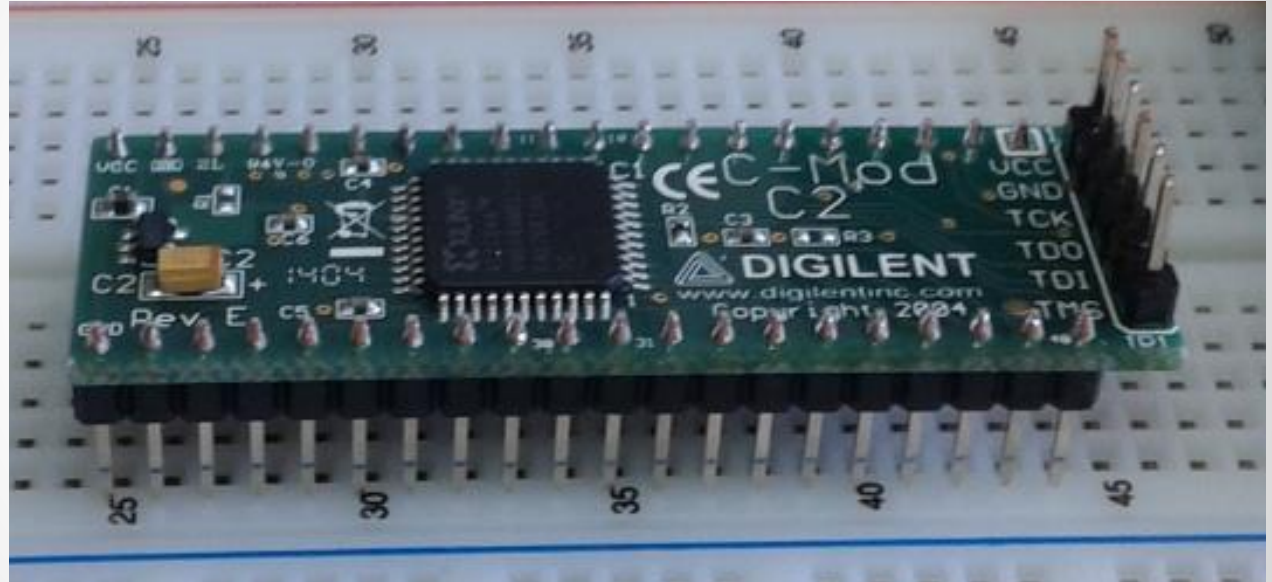
Xilinx XC2C64 in a 2.16 x 0.7 in. DIP package
