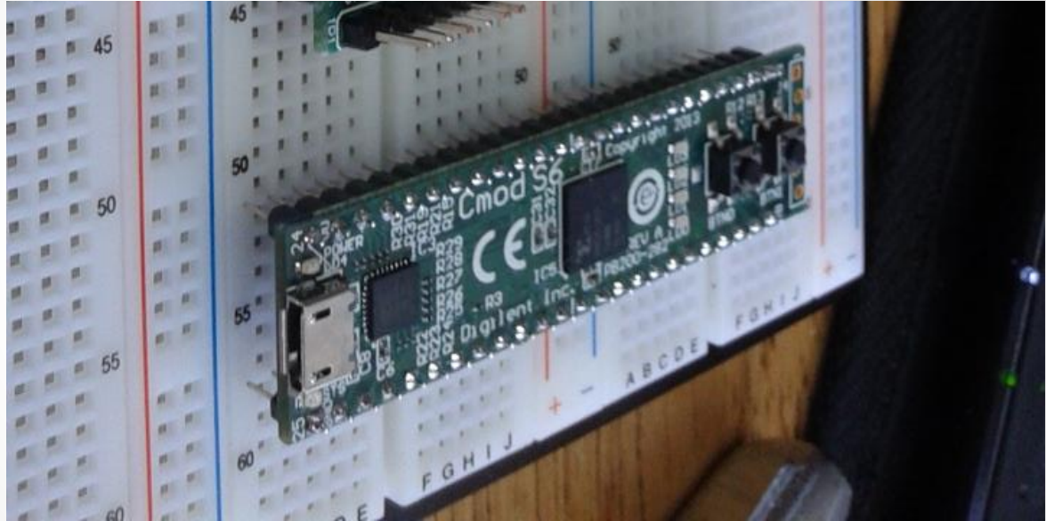
Xilinx XC6SLX4-2CPG196 in a 2.6 x 0.7 in. DIP package
